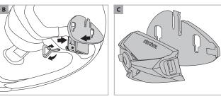
ASSEMBLY OF THE SLIDE SUPPORT WITH REMOVABLE CLIP
