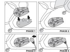
met's finish). Remove the protective film from the double sided tape, and apply the support to the helmet.
