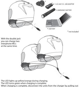
When charging is complete, disconnect the units from the charger by pulling out the jack plug, and also unplug the charger from the outlet.
